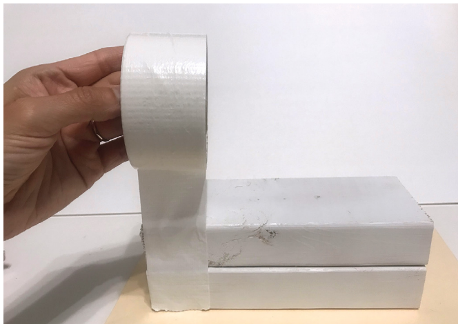
Figure 4 Wrapping the 2" x 4" x 8" Wood Pieces with Duct Tape
